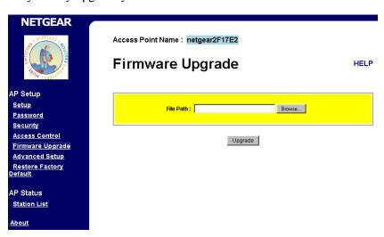
Before upgrading the WAB102 firmware, make sure you have downloaded the latest firmware from the NETGEAR support website: http://www.netgear.com.
